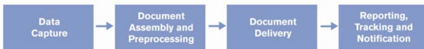
Figure 3: Open Text fax server incorporates a four-phase process that captures information, renders it into an electronic image, distributes the information via fax, email or over the Internet and creates customized reporting, including host notifications.
